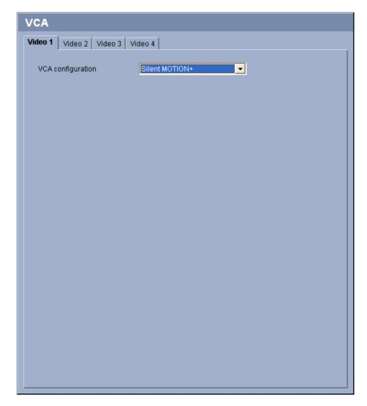
The VideoJet X40 SN contains an integrated video content analysis (VCA), which can detect and analyze changes in the signal on the basis of image processing. Such changes can be due to movements in the camera's field of view.
